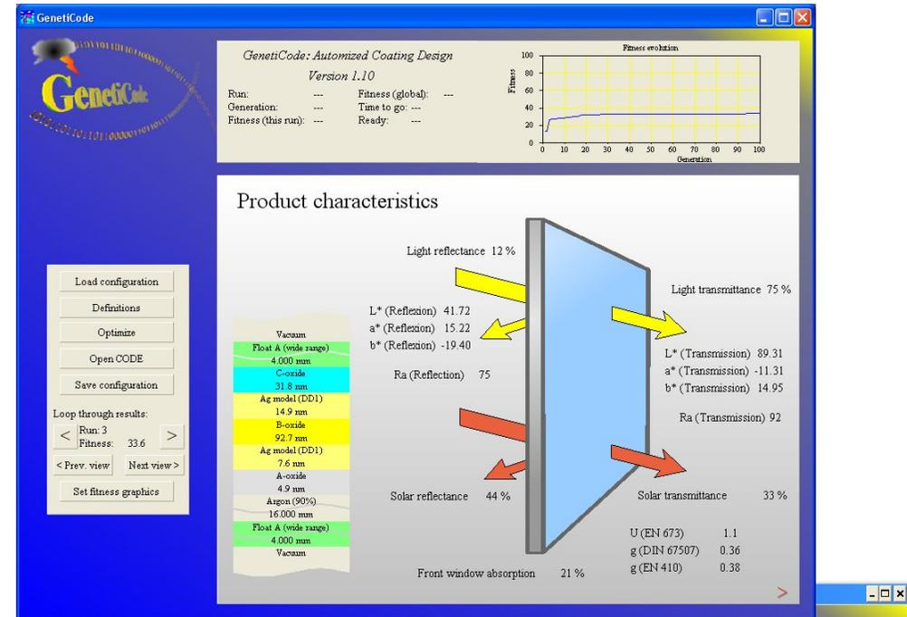
Construction of a band pass filter on glass for 500 nm radiation:
