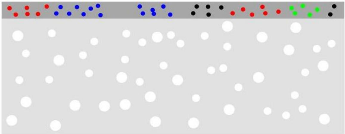
The following steps show how a simple SPRAY model for the simulation of digital prints on paper can be developed. We will consider a circular area of 100  $\mu\text{m}$  radius, fill in some printed dots and compute the total diffuse reflectance of the system.
