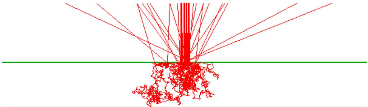
The diffuse reflectance is significantly higher compared to that of the larger inclusions:
