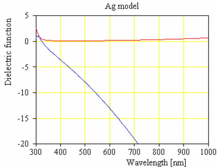
The complex square root of the dielectric function, the refractive index, has an almost vanishing real part and a much larger imaginary part in the case of metals:
