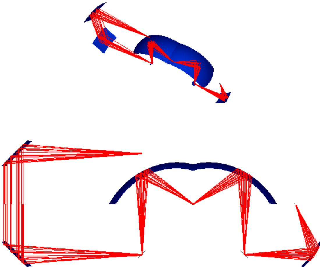
Meanwhile SPRAY has a number of features that turn it into an excellent tool for color prediction. Based on physical modeling, the transfer of light from the light source through light scattering, absorbing and fluorescent media and across partially reflecting interfaces is simulated. SPRAY performs fully three-dimensional ray-tracing with almost no compromises.
