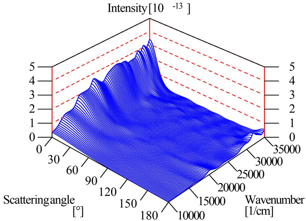
The scattering distribution depends very much on the ratio of the light wavelength and the particle radius. In the infrared (below 15000 1/cm) the ratio is large which leads to a broad angle distribution. In the UV (above 25000 1/cm) the ratio is smaller. Here the distribution is dominated by a strong and sharp forward peak and (weak) backward scattering.
