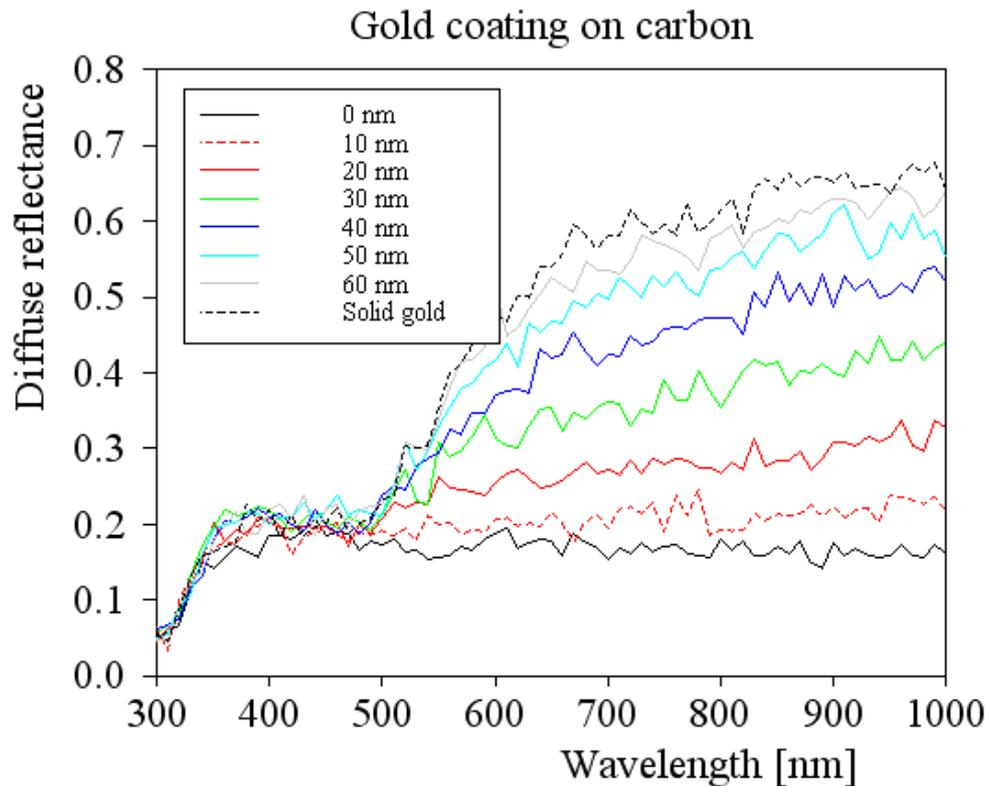
The coating should have a thickness of at least 50 nm. But even at 60 nm thickness the color coordinates are still different from those of a 'solid gold paint'. The latter are indicated by the gray lines in the graph below:
