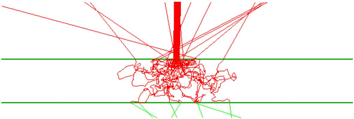
Starting many rays and placing large detectors above and below the paper one can compute the diffuse reflectance and transmittance of the model paper:
