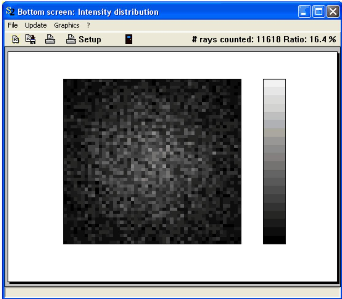
The intensity distributions as well as the diffuse reflectance and transmittance spectra could be compared to measured data in order to estimate how good the model describes the real paper.
