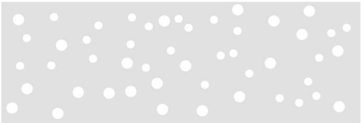
The size distribution of the voids determines the angle-dependence of the average single scattering event (which is computed by the Mie program integrated into SPRAY), whereas the volume fraction of the voids controls the strengths of the scattering, i.e. the scattering coefficient. The host material weakly absorbs in the UV which is controlled by an oscillator term in the optical constant model.
