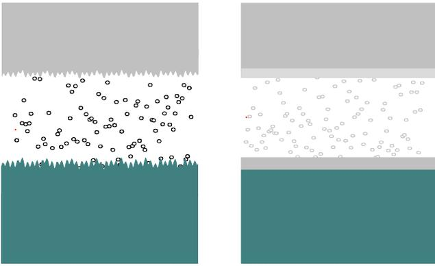
Fig. 3: Schematic sketch of a satisfying silver layer model: The rough interfaces of the 'real' system on the left are approximated by thin effective-medium layers, and the reduction of electron mobility due to diffuse scattering at the rough boundaries is taken into account by an increase of the damping constant in the Drude model.
