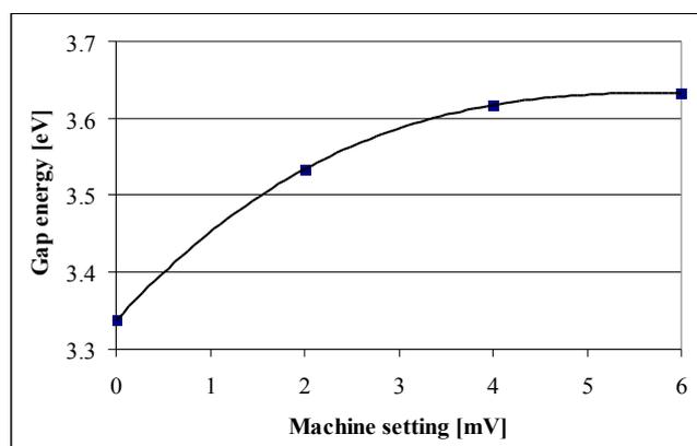
Fig. 1. Example for a simple relation between a deposition parameter (lambda-probe setting) and an optical parameter (gap energy of a reactively sputtered oxide).
