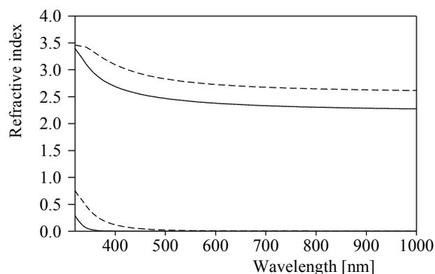
Fig. 2. Optical constants of a reactively sputtered oxide: The upper curves show the real part of the complex refractive index  $n$ , the lower curves the imaginary part  $k$ . The solid lines give the optical constants for 6 mV, the dashed ones for 0 mV.
