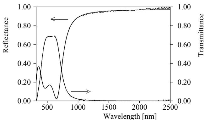
Fig. 4: Simulated (dashed) and measured (solid) spectra of a commercial solar control coating (SEMCO Solar 600) with extraordinary performance: The g-value (according to standard EN 410) of 32% is only 50% of the achieved light transmittance (64%).
