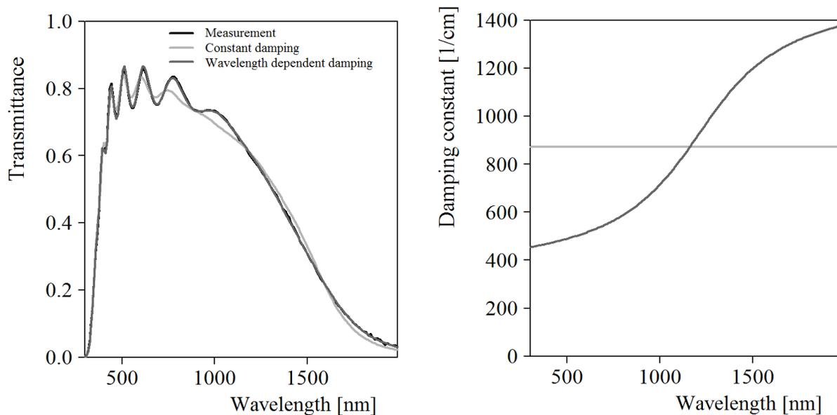
Figure 6. Left: Measured transmittance of a thick (630 nm) ITO layer on glass and two fit results, applying the classical Drude model with constant damping and the extension with wavelength-dependent damping. The values of the damping constants are compared in the right graph.
