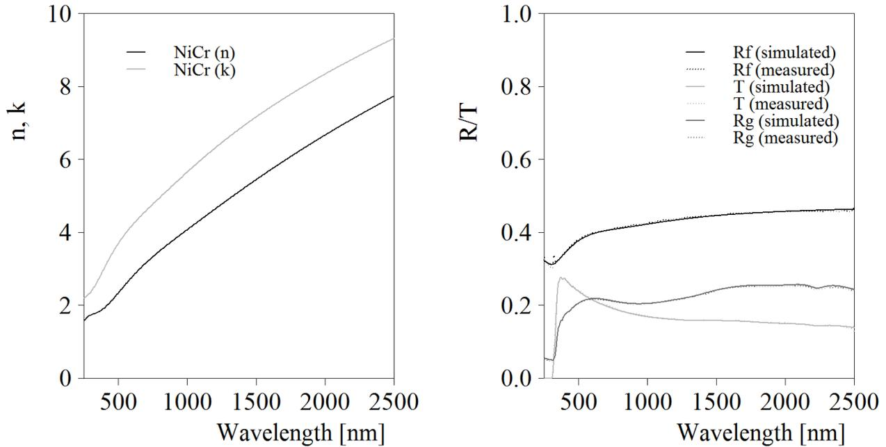
Figure 5. Fit of an optical model for a 10 nm NiCr layer on glass. The complex refractive index obtained by the fit procedure is shown on the left. The sheet resistance of the model perfectly matches the measured value of  $96.8 \Omega$ . The difference between measured and simulated emissivity is small (54.8 % and 52.6 %, respectively).
