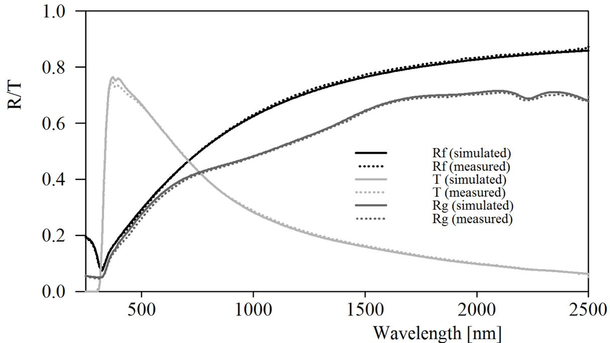
Figure 2. Fit of the optical spectra of a 10 nm silver film on glass, adjusting the electron damping and the film thickness only.
