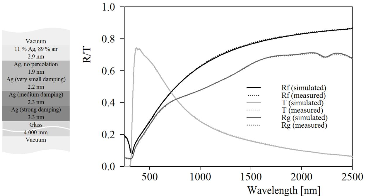
Figure 3. Final optical model which leads to a perfect match of simulated and measured data, including the emissivity of 8.6 % and the sheet resistance of 6.1  $\Omega$ . See text for discussion.
