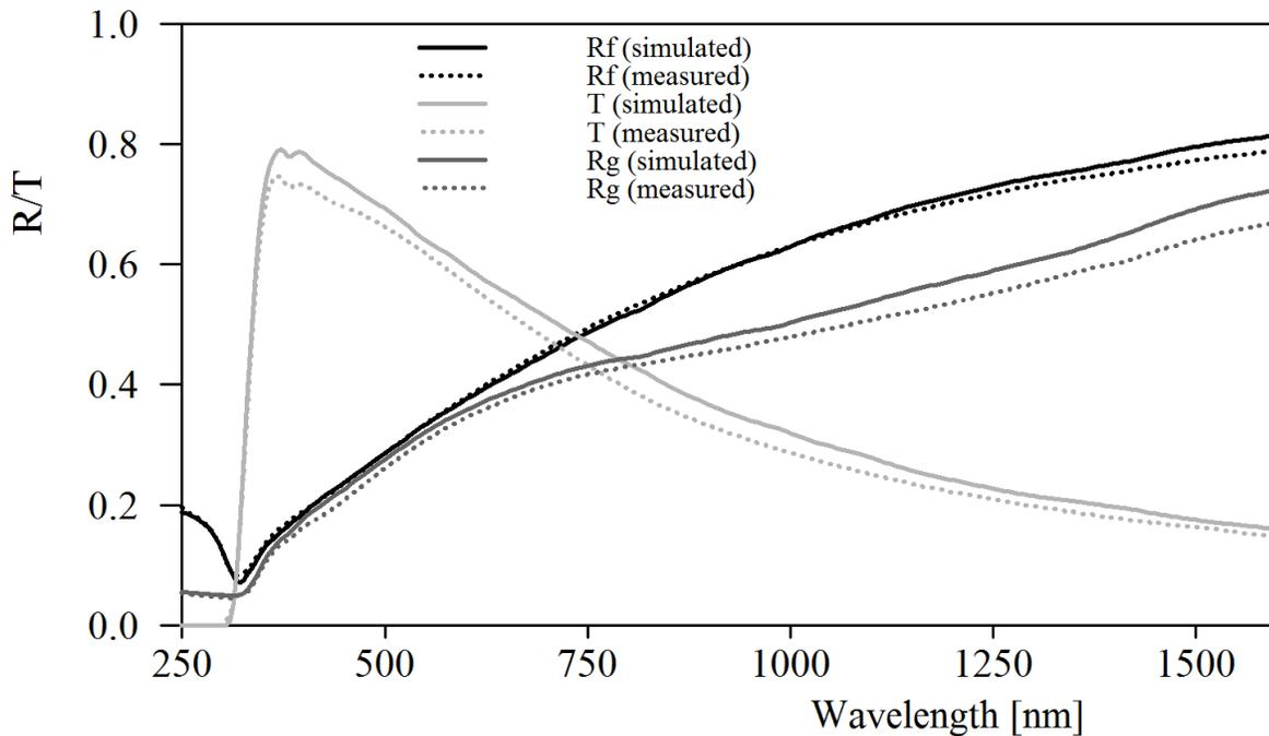
Figure 1. Comparison of measured and simulated spectra, computed using literature data [1] for the optical constants of silver.
