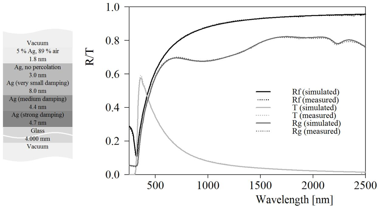
Figure 4. Simulated and measured optical spectra of a 20 nm thick Ag layer on glass. The measured normal emissivity of 3.4 % and the sheet resistance of 2.2  $\Omega$  are perfectly reproduced by this model.
