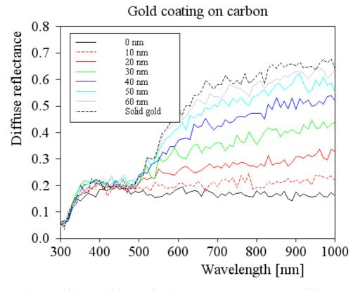
The coating should have a thickness of at least 50 nm. But even at 60 nm thickness the color coordinates are still different from those of a 'solid gold paint'. The latter are indicated by the gray lines in the graph below:
