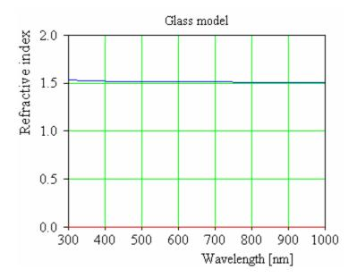
In glasses significant absorption occurs in the mid infrared region (by vibrational modes) and in the far UV (by optical interband transitions). Due to the large electronic bandgap in these types of material the visible spectral range is almost absorption-free.
