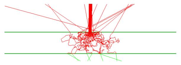
Starting many rays and placing large detectors above and below the paper one can compute the diffuse reflectance and transmittance of the model paper:
