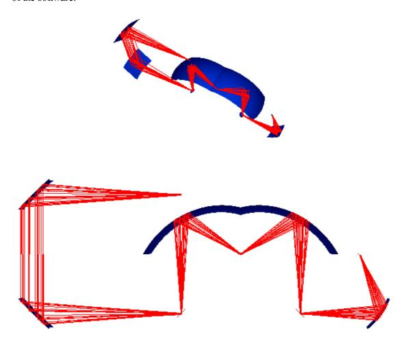
Meanwhile SPRAY has a number of features that turn it into an excellent tool for color prediction. Based on physical modeling, the transfer of light from the light source through light scattering, absorbing and fluorescent media and across partially reflecting interfaces is simulated. SPRAY performs fully three-dimensional ray-tracing with almost no compromises.
