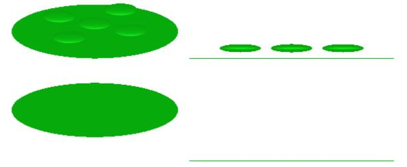
The dots are embedded in a homogeneous layer with a thickness of  $15~\mu m$ . A circular transparent light source is set directly above the top surface. It illuminates the sample from the top with Lambertian characteristics. Around the scenery we have placed a cylindrical ideal mirror which introduces reflecting boundary conditions:
