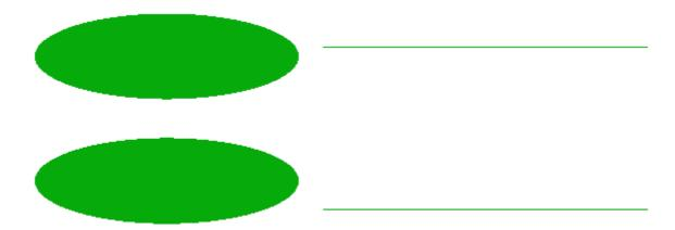
The dots are modeled by flat ellipsoids which are filled with pigments. The volume fraction of the pigments inside the dots is 5%, the dot diameter and height are 40  $\mu$ m and 8  $\mu$ m, respectively:
