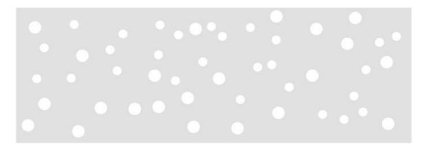
The size distribution of the voids determines the angle-dependence of the average single scattering event (which is computed by the Mie program integrated into SPRAY), whereas the volume fraction of the voids controls the strengths of the scattering, i.e. the scattering coefficient. The host material weakly absorbs in the UV which is controlled by an oscillator term in the optical constant model.
