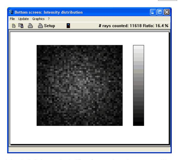
The intensity distributions as well as the diffuse reflectance and transmittance spectra could be compared to measured data in order to estimate how good the model describes the real paper.
