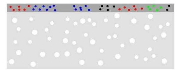
The following steps show how a simple SPRAY model for the simulation of digital prints on paper can be developed. We will consider a circular area of  $100~\mu m$  radius, fill in some printed dots and compute the total diffuse reflectanc of the system.
