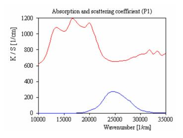
Sorry, all scattering properties are displayed in SPRAY using wavenumbers. Wavenumbers are inverse wavelengths measured in cm (i.e. 1/cm). 10000 1/cm correspond to 1000 nm wavelength (near infrared), 25000 1/cm are 400 nm (blue end of the visible). Note the rich structure in the scattering probability which depends on the sphere size distribution. The rays scattered by pigment P1 get new directions according to this distribution:
