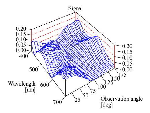
The observed features are interference effects which depend on the angle of observation, of course.
