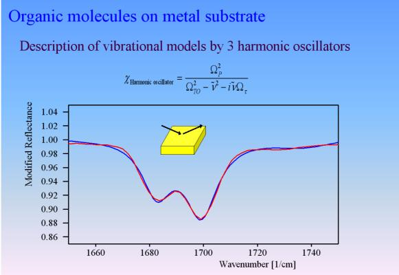
Extensions of the harmonic oscillator model are required if the line shape is not a Lorentzian. With a fourth oscillator parameter, the so-called Kim model (shown below) can describe both Gaussian and Lorentzian line shapes of absorption bands, and any lineshape in between these two extremes.
