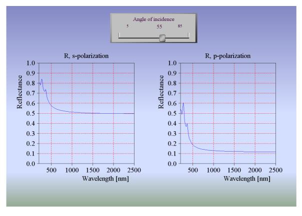
A similar simple test for correct reflectance and transmittance measurements can be done with conventional microscope slides. The measured spectra should not differ from the simulated ones by more than 1 or 2 percent:
