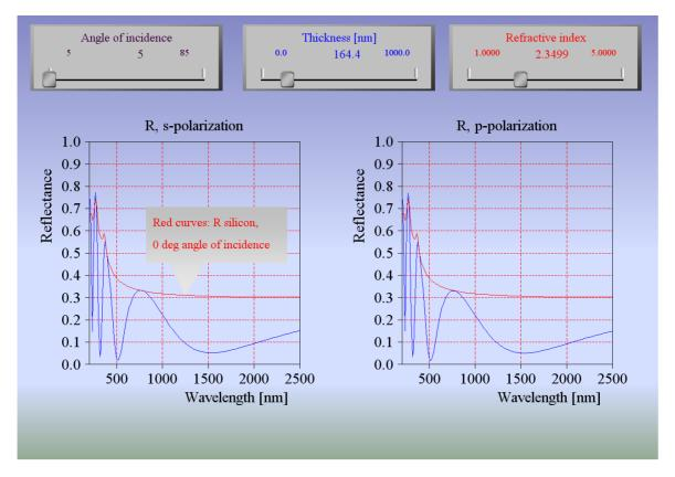
The phase shift  $\phi$  leads to interference fringes in the case of a transparent layer:
