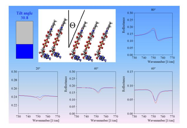
Here is a real case of molelcular orientation analysis: For a layer of perylene molecules on a Si wafer the reflectance spectra taken at several angles of incidence are fitted simultaneously. For each vibrational mode the orientation angle with respect to the surface normal of the Si wafer could be determined. From the angular information the absolute orientation of the molecules was finally deduced.
