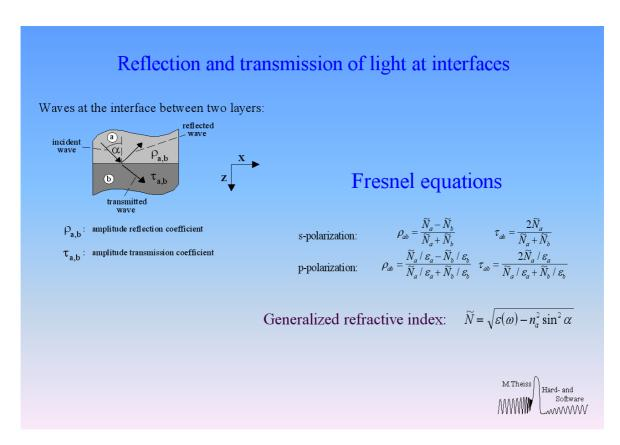
In the case of a single layer between two 'halfspaces' the total reflected and transmitted waves are the sum of many partial waves. The summation can be done conveniently making use of a geometric series:
