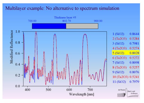
The increase of one of the layer thicknesses (layer 5, marked yellow) by 10 nm leads to complicated variations of the spectrum which can only be handled by a reliable physical model:
