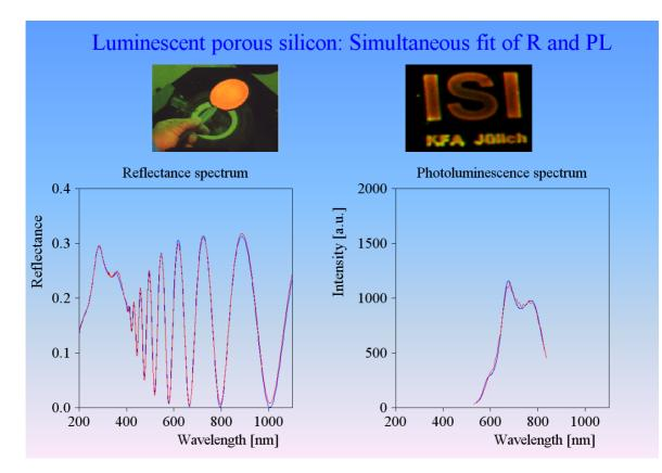
In the case of multiple spectrum fits each spectrum should have an individual weight for the computation of the total fit deviation (i.e. the difference between measured and simulated spectrum).
