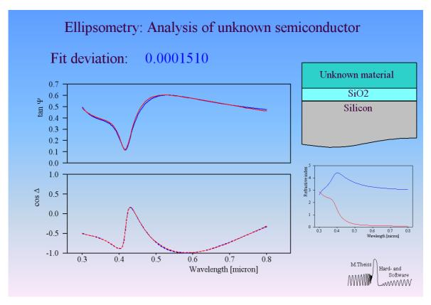
The fit can be improved introducing a thin surface layer which represents surface roughness. The layer is an effective medium mixture of the unknown material and air. The obtained optical constants differ not very much, but significantly from the ones obtained without surface roughness. In important cases the assumption of the existance of a surface roughness should be confirmed by an independent method such as AFM.
