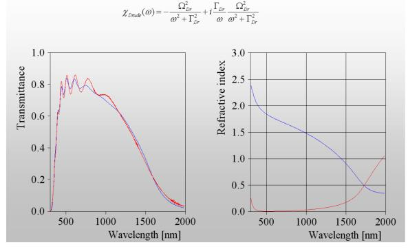
An extended Drude model with a (still quite simple) frequency dependent damping constant leads to a significant improvement of the fit with much more reliable results for the film thickness and the other model parameters such as gap energy and resistivity:
