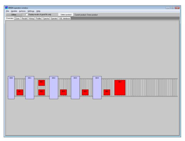
A mouse click on an object pops up a dialog showing the object's parameters that can be changed. The most important objects are the deposition devices and the bright eyes. Clicking on a deposition device brings up the following dialog:
